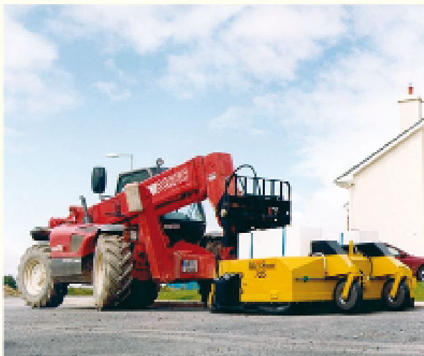
Model 725 complete with gravity water system powered off the hydraulic service of the material handler.
