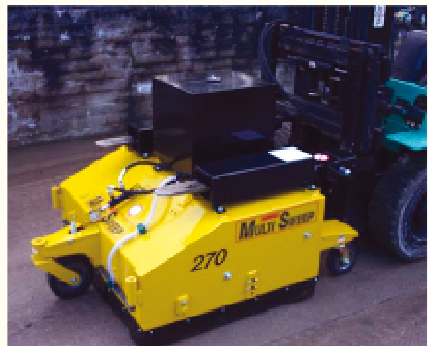
Model 270 complete with single tank gravity water system and powered off the hydraulics of the forklift.
