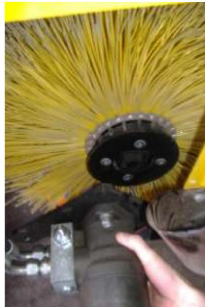
11: Once the motor has been removed from the drive shaft, it can hang from its hydraulic hoses. At this stage you can begin to lift the MultiSweep up and away from the broom. Please ensure as you are lifting that the broom is complete free from the MultiSweep.
