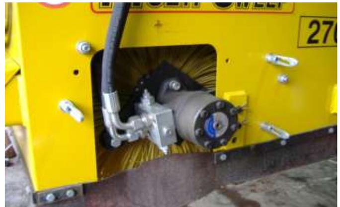
5: Once the “barrels” take the weight of the broom, unclip the adjustment blocks on both sides of the MultiSweep (V183).
