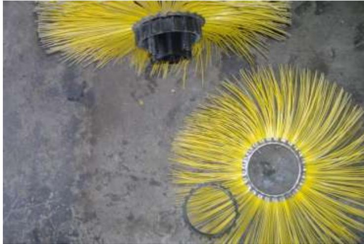
14: Slide one spacer (B129) on from the motor side, followed by a poly (B160) section, then a spacer, then a wire section and spacer and so on. There is a pin on each poly/wire section that lines up with a track on the mandrill.
