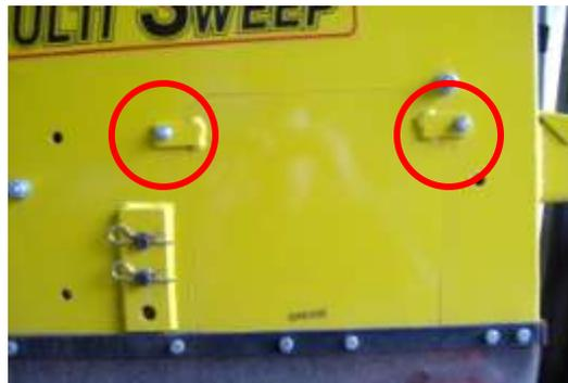
7: Next unbolt the four anchoring points of the broom (2 on either side of the sweeper F103, F202), be careful not to lose the two bushings (V116) from the bearing and motor arms.
