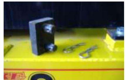
6: Remove the side plate from the bearing side of the MultiSweep. This is done by unbolting the 2 M8 nuts and bolts.
