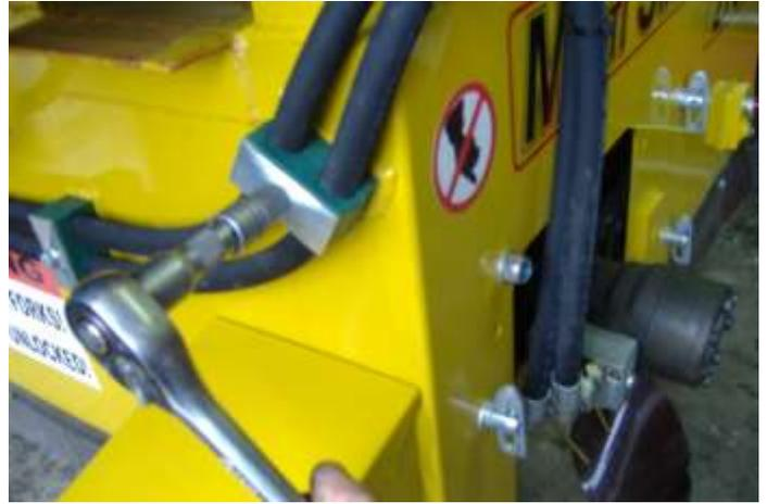
9: Now Lift the sweeper slowly with your forklift, until the motor arm (V188) is clear of the side wall.
