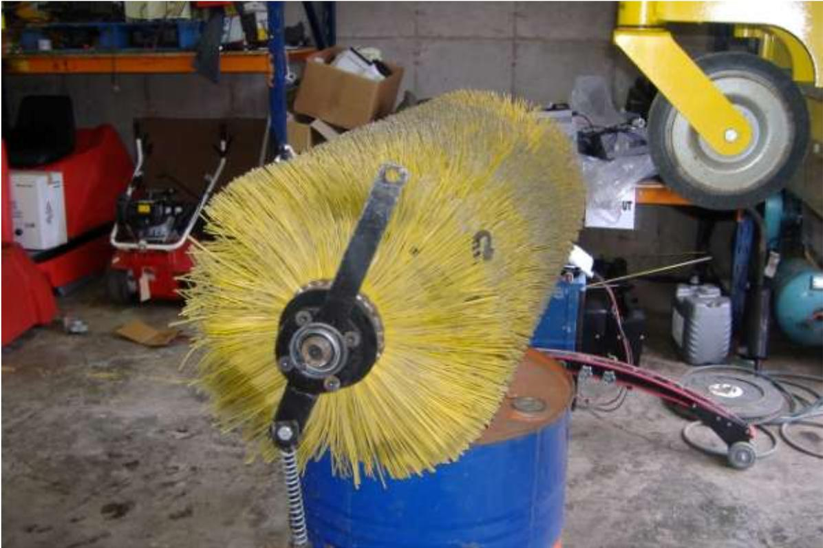
12: Now it is time to unbolt the four counter sunk allen head bolts (F160) from the end plate (B122) on the motor side, as below.
